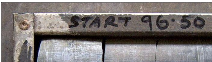
Figure 1 Label the starting depth of the cored interval on the top left corner of the tray
