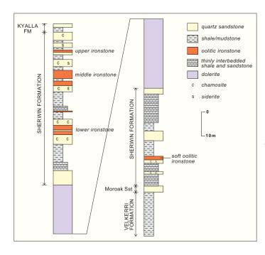
Stratigraphic section representative of the Roper Valley area (based on drillholes BHP DDHB7 and BMR Urapunga DDH4).
